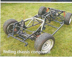
Rolling chassis completed.
